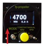
In this mode, the system adjusts the pitch completely automatically based on the MDP-RPM TARGET curve inserted in the microcontroller for the selected engine. The setting range for Rotax engine ranges from 4000 to 5500 RPM (5800 RPM in takeoff mode, please check chapter 7 for other modes)
