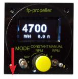
In this mode, the pilot decides the target RPM by turning the potentiometer (B) and the governor moves the propeller pitch to reach that target value.
